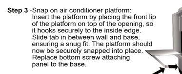
Tab must be fully inserted to the bend
